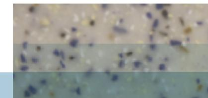
Fine sanding is completed using the 3M 443SA Trizact Disc P3000. These steps reduce surface roughness and minimize the following polishing process. Finally the 3M Finesse-it Finishing Material and 3M Finesse-it Buffing pad (Lambs wool) are used together to polish the surface.
